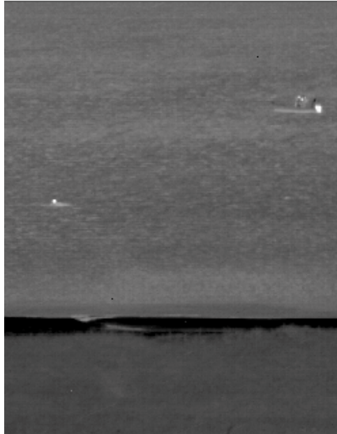
Figure 8: IR Images of Swimmer (lower-left) and RHIB (upper-right)
