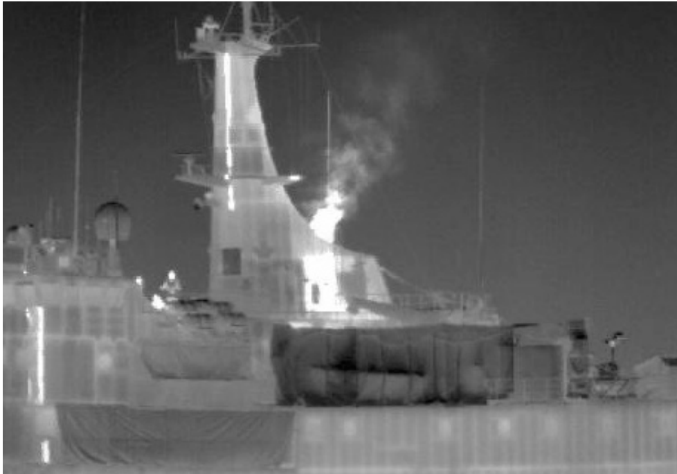
Figure 5: Short-Range IR Image of the Starboard Diesel Plume.
