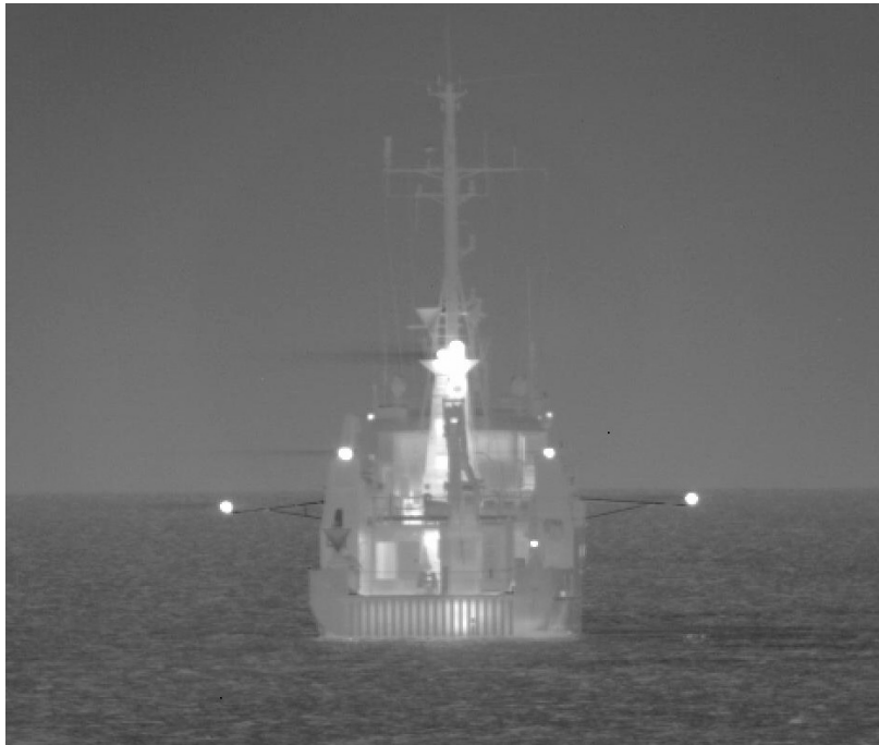
Figure 9: IR Image of Mittlegrund Showing IR Sources.
